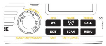
Close-up of the Link-5 base station radio, showing the keys
